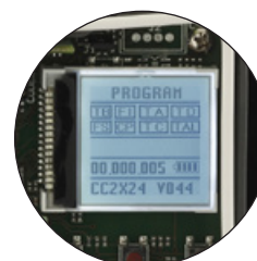
SELF-PROGRAMMING MONITORED BY AN LCD GRAPHICS DISPLAY CC242ETOPCB - CC242EXTOPCB
